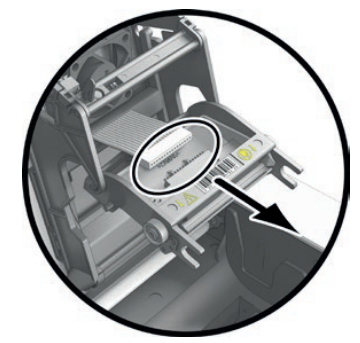
4 Tilt the head carefully downwards and disconnect the connector linked to the cable without forcing the mechanism.
