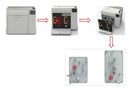
Warning: When card printer shipped from the factory, there will be placed a piece of sponge paper next to the print head, please take it off before use or the power on test, otherwise it may cause damage to the printhead. Operation steps are as follows. As shown in the picture below, follow the operating guidelines to remove the right ribbon holder, and then remove the sponge paper as shown.
