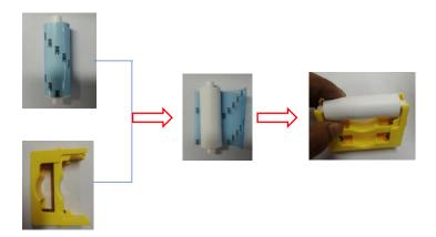
After tearing off the 3M adhesive layer, hold the two ends of the cleaning roller with your hands, push them to the installation position and gently press down to lock the two ends of the cleaning roller.
