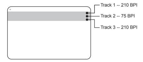
Each track can be encoded and decoded with ASCII characters in the standard default ISO data formats:
