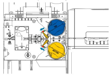
**Step 3.** Rotate each cassette in the direction indicated below until it stops.
