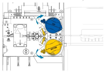
**Step 4.** Remove each cassette by pulling straight out from its spindle.
