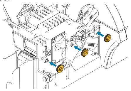
In some cases, a card may get wrapped around the laminator heater assembly rollers. In this case, the laminator heater assembly can be removed.
