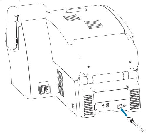
**Step 2.** Insert the opposite end of the Ethernet cable into an appropriate Host port.
