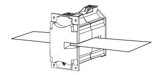
**Step 9.** Remove the card from the heater assembly.
