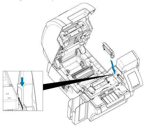
**Step 3.** Press down on the cartridge until it is fully seated.
