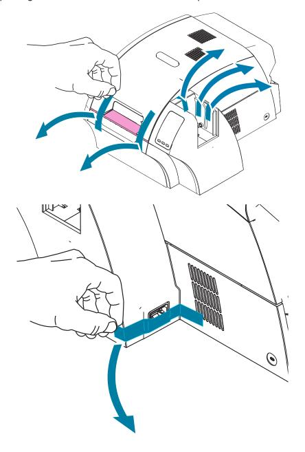
Then, open the printer by pressing the yellow release button and remove the packing material.
