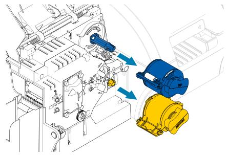
**Step 5.** Open each cassette by separating its two halves at the hinge—grasp the two halves firmly then pull apart. **DO NOT use tools**.
