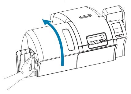
**Step 2.** Unlock the laminate cassette by rotate the locking lever in the direction indicated.
