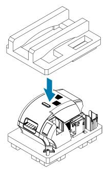
Step 13. Roll up the power cord and USB cable and place them in the recess of the upper foam insert.
