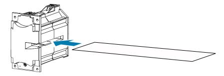
**Step 8.** Pull the card all the way through the heater assembly thereby cleaning the heater rollers.
