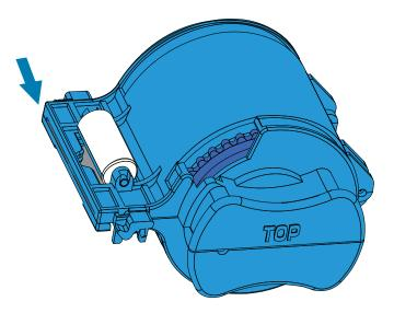
**Step 6.** Install the cassette—see Installing the Laminate Cassette on page 21.
