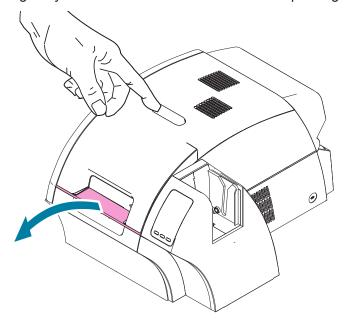
If the printer came with the optional laminator installed, remove the packing tape from the laminator.
