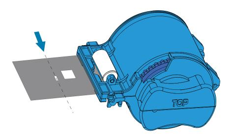
**Step 5.** Rotate the core to adjust the laminate overhang. Stop when the end of the laminate (not the edge of the index hole) is even with the edge of the lips of the cassette.
