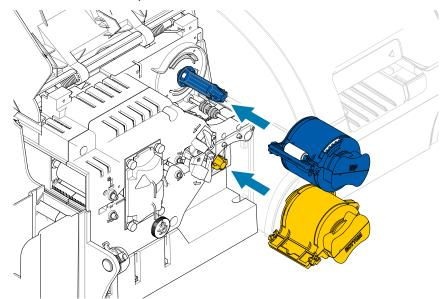
**Step 3.** Rotate each cassette (in the direction indicated in the figure below).
