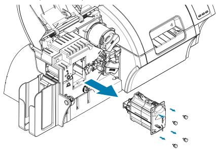
**Step 2.** Remove the card—do not use tools. If the card is wrapped around the heater assembly rollers, contact Zebra to replace the heater assembly.
