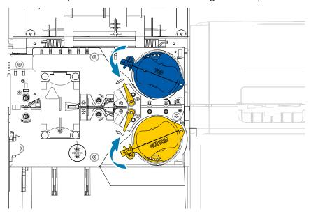
**Step 4.** Continue to turn the cassette. The locking lever will move to the left as the cassette rotates over the locking mechanism, and will then click into the locked (green) position.
