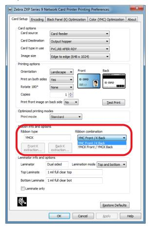
In the example above, the available ribbon combinations for the installed YMCK ribbon are YMC on the front of the card, and K on the back of the card; or YMCK on both the front and back of the card. The available Ribbon combinations is also dependent on if printing is set to single- or double sided.
