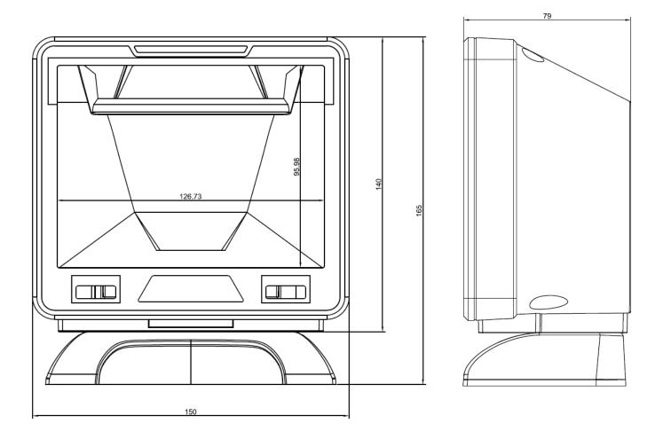
Without stand, size is 150\*140\*79mm, 421g(not include cable) With stand, size is 150\*165\*79mm, 480g(not include cable)
